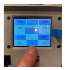
This screen is used to control the unit. Here you can turn on the pump, input model name, tank size in milliliters and switch to the manual pump screen.
